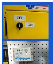
To change the batteries on an INSTABOOM, switch off the barrier with the power switch on the side, then open the cabinet and press the button on the regulator once so the Load light goes off.
