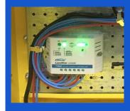
Press and release the button on the solar regulator until the Load light illuminates and then close the cabinet. Turn on the barrier for initial setup and test.
